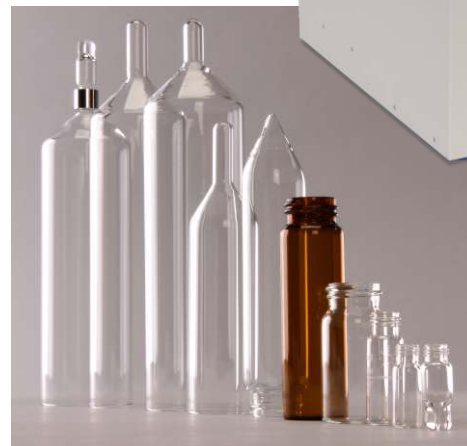
Measurements - Concentration / Evaporation vessels in 500 µL, 1 mL, and direct to a GC Vial or to dryness
